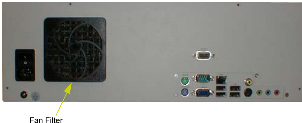
Figure 12 Server Module Fan Filter
